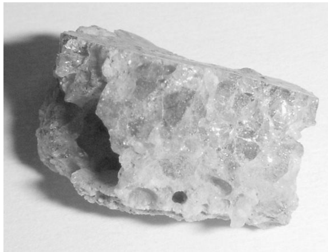
FIGURE 4. Trinitite, an entirely new mineral formed by the explosion of the Gadget, the first nuclear device. Photograph by Shaddack.
